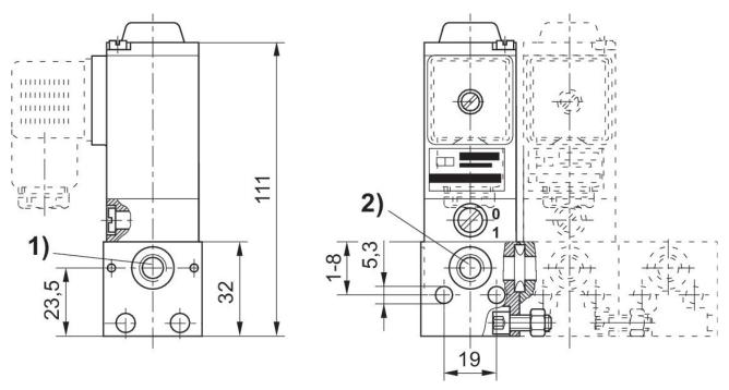
Scope of delivery: 2 screws M5x12, 2 nuts M5 DIN 934, 1 O-ring 1) Port 1 (Input) 2) Port 2 (Output)
